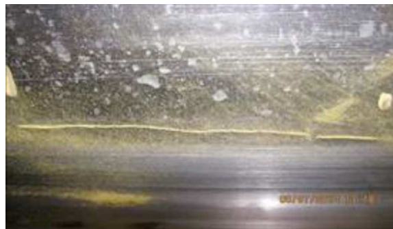
FIG. 3 Two Cracks on Tooth Just Above the Root cracks on a tooth just above the root that were only observed visually after being revealed by the ECA examination. In this example, the cracks were not apparent visually until MT was performed.
