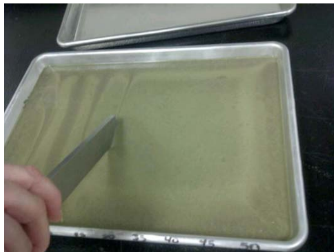
FIG. 1 Full-Depth Cut in Test Specimen
