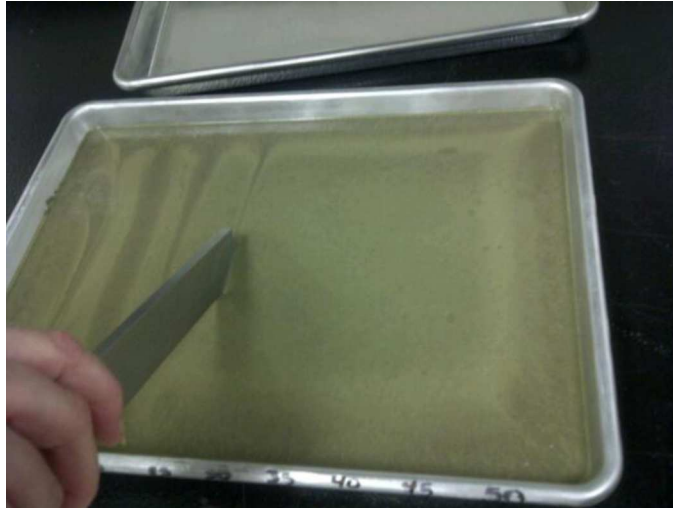
FIG. 1 Full-Depth Cut in Test Specimen
