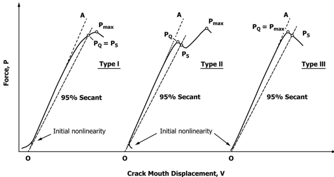
FIG. 7 Principal Types of Force-Displacement (CMOD) Records
