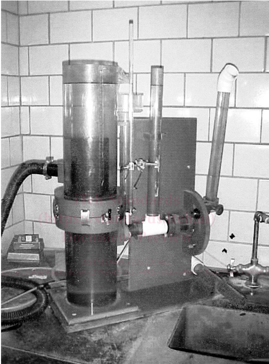
FIG. 1 Constant and Falling Head Permeability Apparatus
