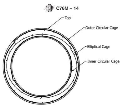
NOTE 1—The total reinforcement area of the inner circular cage and the elliptical cage shall not be less than that specified for the inner cage in Tables 1-5.
