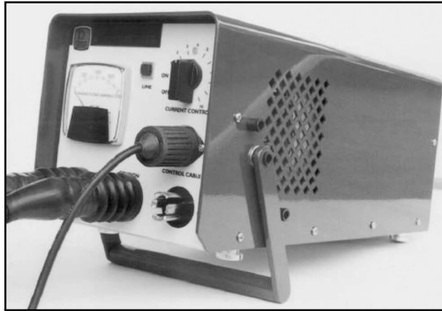
Typical portable power pack for prods
