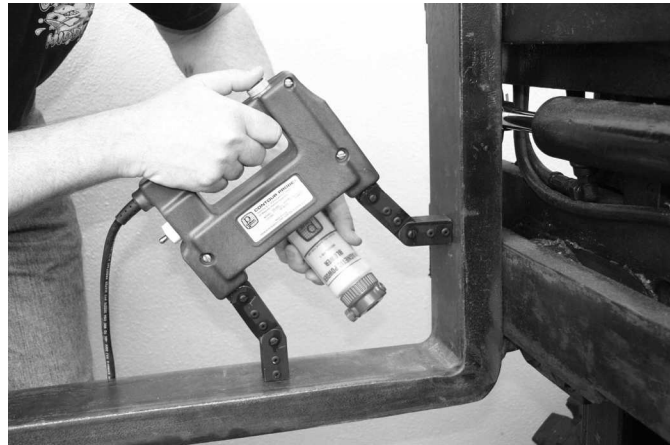
FIG. 1 Yoke Method of Part Magnetization
