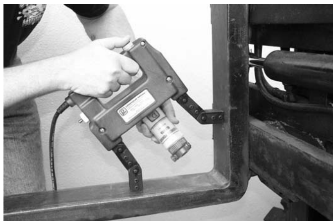
FIG. 1 Yoke Method of Part Magnetization
