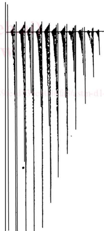
FIG. 12 Sample Drum Record of Impact Bending Test
