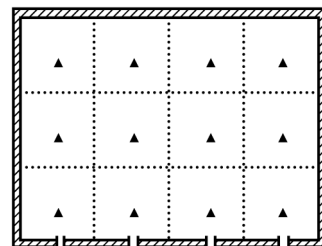
FIG. 1 Traverse Positions for Rectangular Flue
