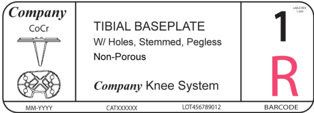
FIG. 3 Another Visual Representation of Guide Using ISSL as Primary Identifier on the End of the Box
