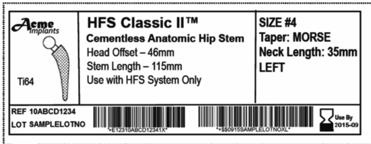
FIG. 2 Visual Representation of Guide Using ISSL as Primary Identifier on the End of the Box
