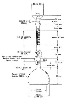
Note 1—Variations of a few millimetres in such dimensions as total height of flask, diameter of base, and so forth, are to be expected and will not be considered sufficient cause for rejection. The dimensions of the flask shown in Fig. 1 apply only to new flasks and not to flasks in use which meet the other requirements of this test method.
