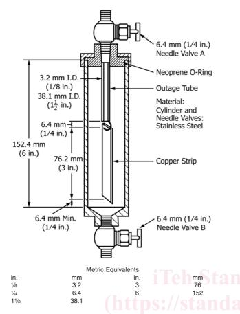
FIG. 1 Copper Strip Corrosion Test Cylinder
