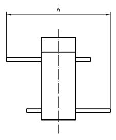
NOTE It is assumed, for this measurement, that the vehicle is standing on a horizontal surface.
