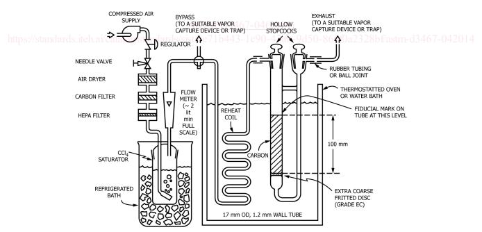
Note 1—These items for the apparatus are critical: the dimensions of the sample tube; the location of the flowmeter downstream of the  $CCl_4$  saturator; and the location of the stopcocks. Reheat coil must be adequate to bring the gas temperature to within  $1^{\circ}C$  of the water bath temperature (that is, bed temperature).
