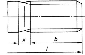
**Fully threaded screws – Distance of the last full form thread from the bearing area**
