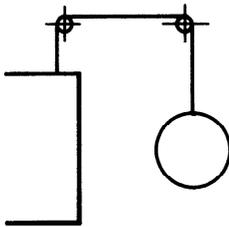
**6.2.5** Tank gauge-float type, top-mounted
