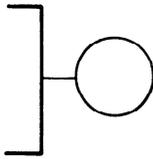
**6.2.3** Instrument with two connections, for example external displacer type
