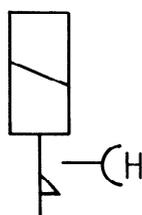
6.4.7 Solenoid actuator with reset (remote electrical)
