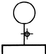
**6.2.6** Level control valve — mechanical linkage
