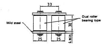
Figure 1 : Peel test fixture for supporting test specimen
