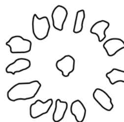
FIG. 2 Typical Injector Spray Pattern
