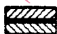
Figure 3. Lap joint test piece with thick bond line (angle between growth ring surfaces and surfaces to be bonded = 30^\circ to 90^\circ )
