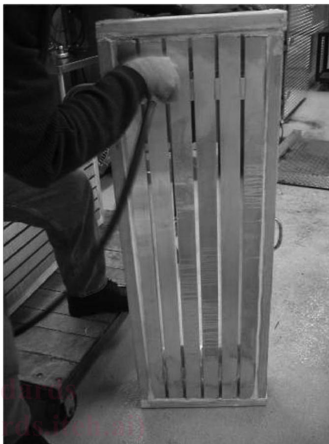
FIG. 1 An Assembled Test Jig Apparatus Ready for Joint Filling with a Perimeter Seal Applied in the Wood Test Buck
