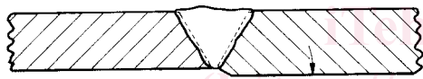
FIG. 15 Butt Joint, Socket Weld to Socket Weld Valve, Fitting or Flange Welded on Pipe Nipple
