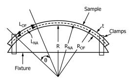
R = radius of jig R<sub>NA</sub> = radius of neutral axis
