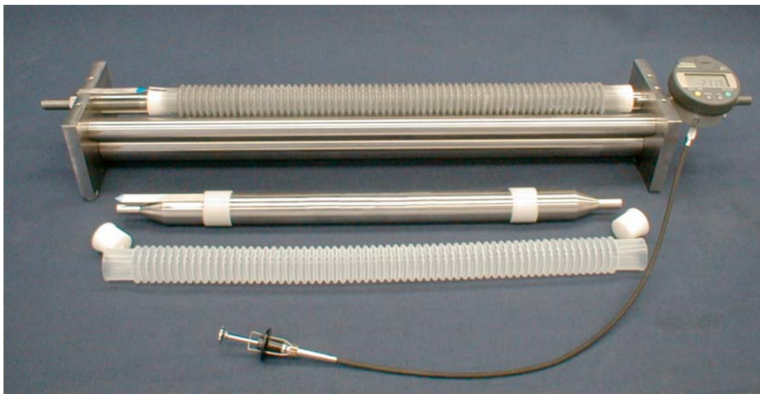
NOTE 1—In the foreground a corrugated PE-mold with two specially shaped end plugs and a 425 mm reference bar. In the background the dilatometer bench with a test specimen placed for length measurement. To the right a digital length gauge with remote control.
