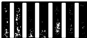
FIG. 3 Stroboscopic Lines Opening When Timer is Adjusted to Exactly 200 r/min
