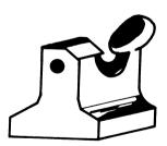
**3.3.2** Unit loads with a flat base area the dimensions of which are less than the overall dimensions (for example: conical tanks with projecting side parts such as handles, rims, etc., or conveyed product wider than the container or pallet, etc.)
