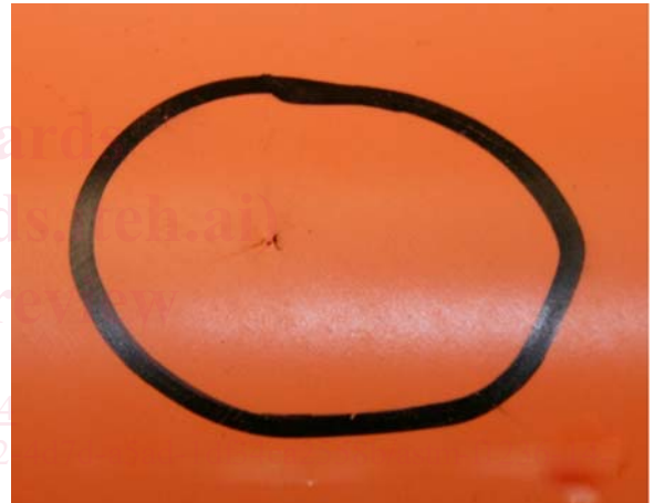
FIG. 5 Breakdown (Dielectric Failure Blanket: Front)
