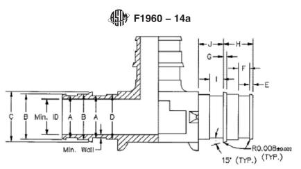
NOTE-BREAK ALL INTERNAL CORNERS .003-min ALL DIAMETER CONCENTRICITY .005 TIR
