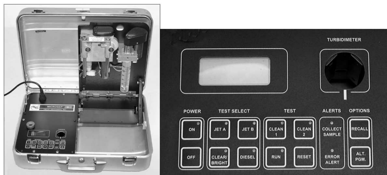
FIG. 2 Micro-Separometer Mark X and Control Panel
