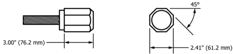
FIG 3B: BLUNT IMPACTOR FIG. 3 Blunt Impactor Assembly
