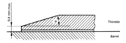
FIGURE 2 - Distance from barrel to graduated face of thimble
