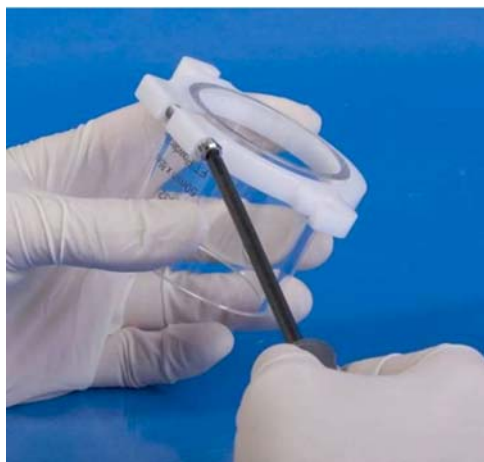
FIG. 5 Fitting the Clamp Ring
