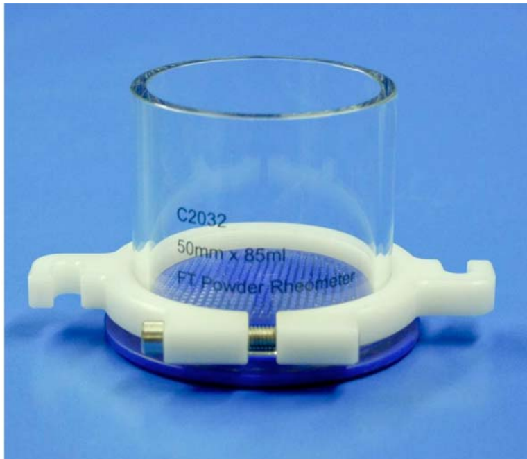
FIG. 6 Fitting the Serrated Base
