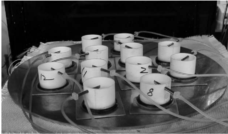
FIG. 3 Test Coupons on Hot Plate
