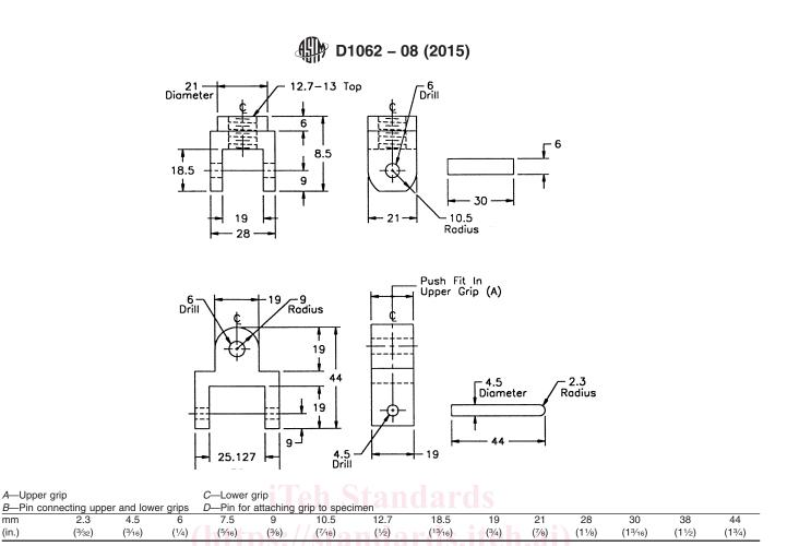
FIG. 1 Details of Test Grips
