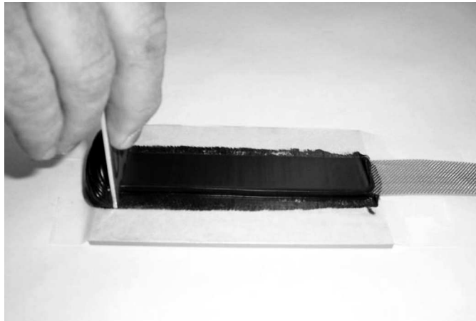
FIG. 7 Tooling Second Bead of Sealant with Special Tooling Device – Side B
