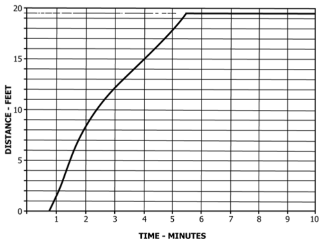
FIG. 7 Representative Time-Distance Curve for Flame Spread of Red Oak
