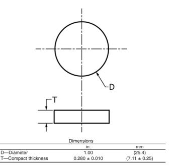
FIG. 1 PM Cylindrical Powder Compressibility Test Specimen
