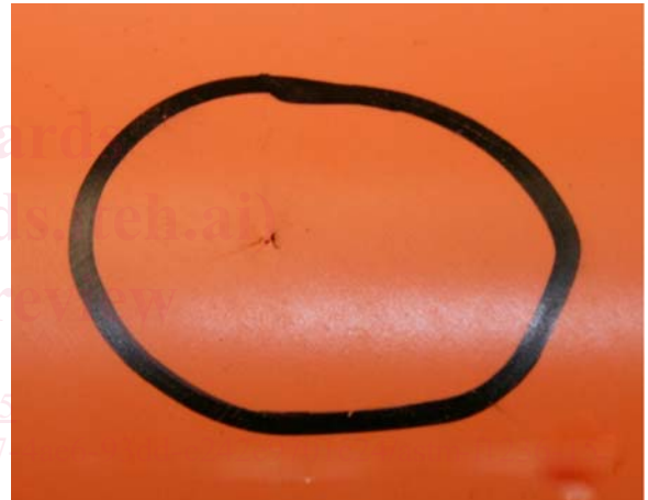
FIG. 5 Breakdown (Dielectric Failure Blanket: Front)
