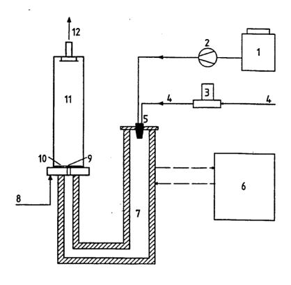
1 DEHS tank 7 Vapourisation pipe with heater and insulation
