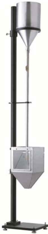
FIG. 1 Apparatus for Falling Sand Abrasion Test
