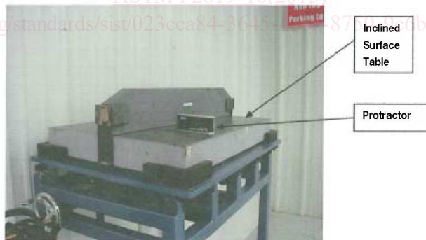
FIG. 5 Example of Inclined Surface Table and Protractor Used to Measure Straightness by the Roll Test Method
