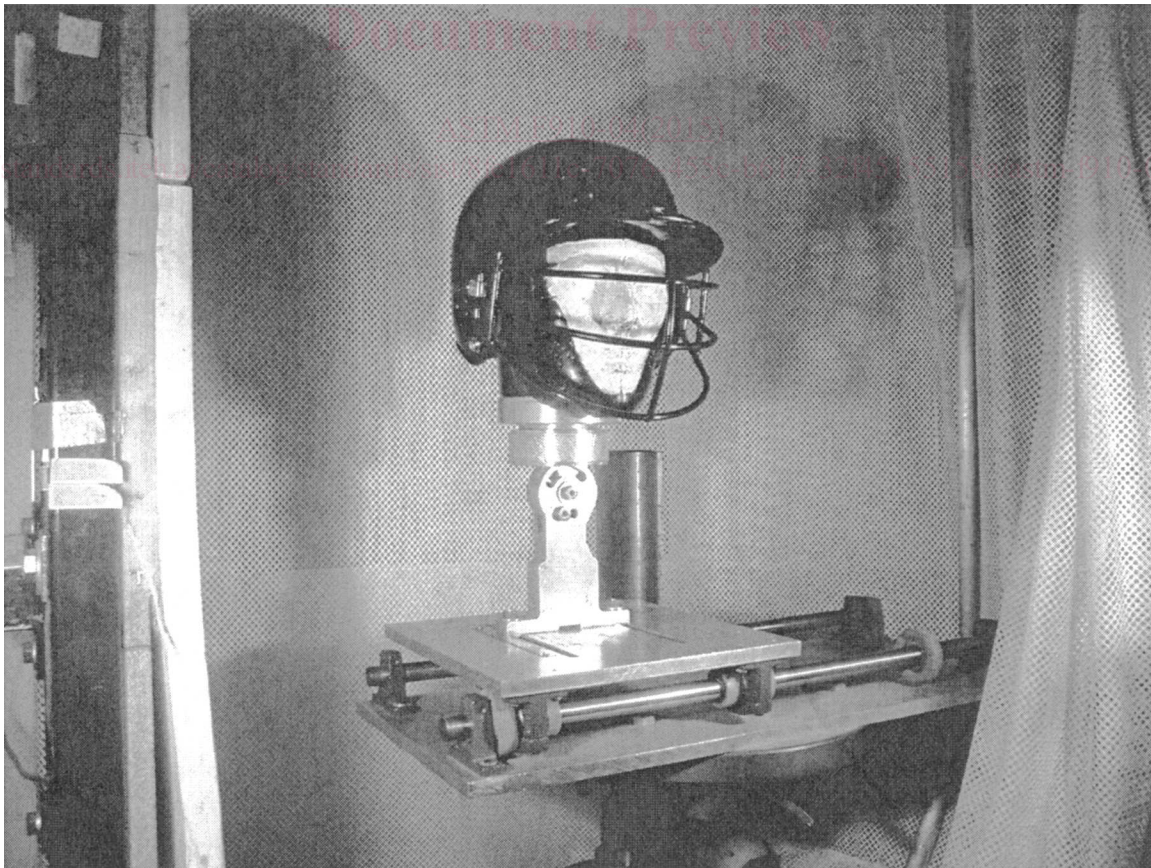
FIG. 1 Face Guard and Helmet on Headform
