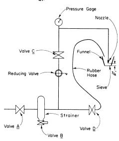
NOTE 1—Industrial/O.E.M. filter and pleated polyester fabric reusable cartridges have been found to be a satisfactory strainer.<sup>4</sup> NOTE 2—Corrosion-free piping must be used.
