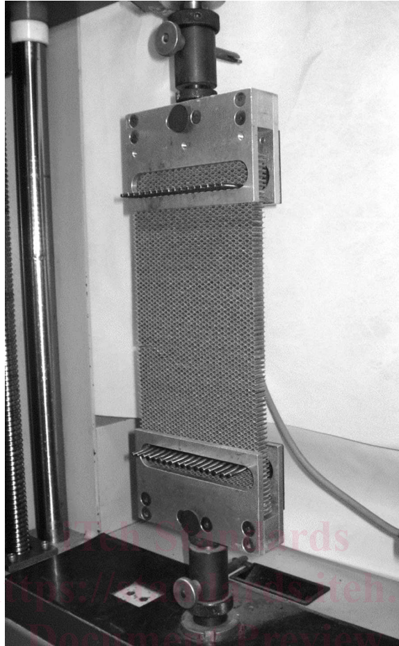
FIG. 1 Honeycomb Core Tensile-Node Bond Strength Test Setup
