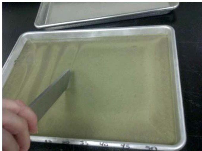
FIG. 1 Full-Depth Cut in Test Specimen
