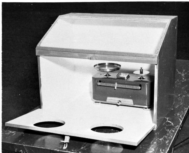
FIG. 1 Weighing Box and Balance
