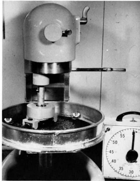
FIG. 43 Specimen in Place Ready for Test (C-100 machine pictured)
