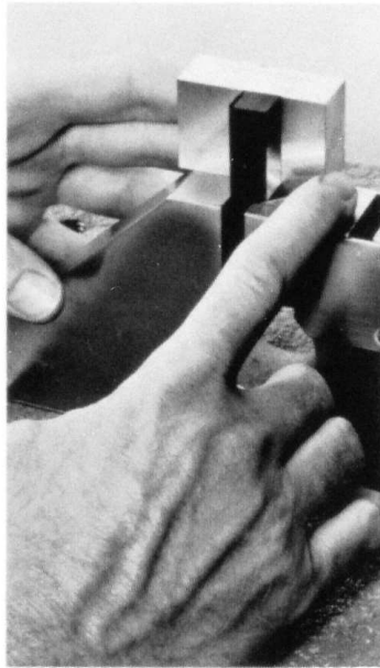
FIG. 4 Jig for Positioning Specimen for Clamping
