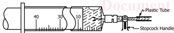
FIG. 2 Conditioning of Syringe, Stopcock Handle in Line with Flushing Port
