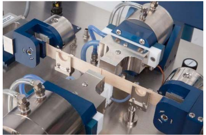
A typical test sample mounted in an apparatus for rapid bond heating and pressing followed by bond pulling.
