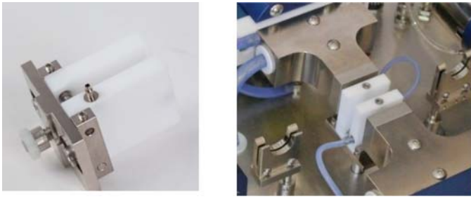
An attachment for rapid air-jet cooling which may be raised, activated and lowered automatically.
